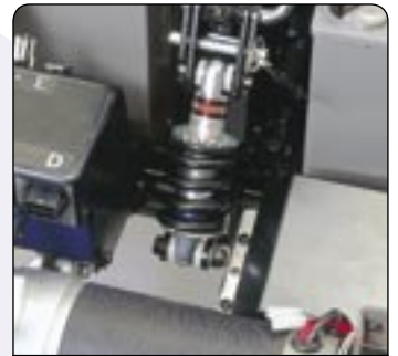
Auriga 10 Spring suspension Adjustable according to individual preferences
