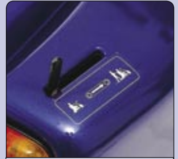
Disengaging lever Disengage the motor brake to enable manual manoeuvring
