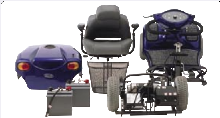
Disassembling No tools are required to dismantle the Invacare® Auriga
