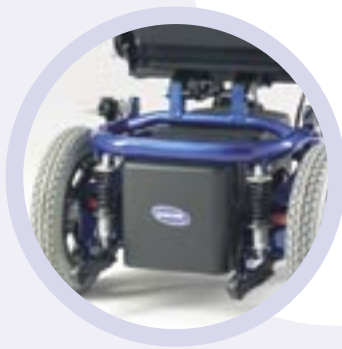
Rear wheel suspension for better shock absorption.
