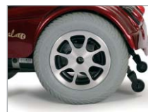
Robust 14" rear wheels for superb traction
