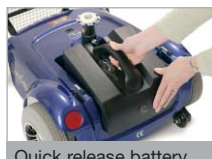
Quick release battery pack for convenient offboard charging
