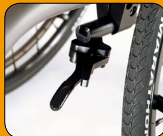
Compact wheel lock folds away nicely below the frame
