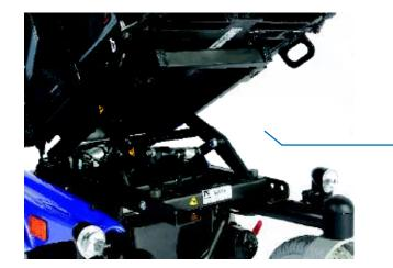
Powered tilt module (0° to 30°) with centre of gravity adjustment to suit correct users balance.
