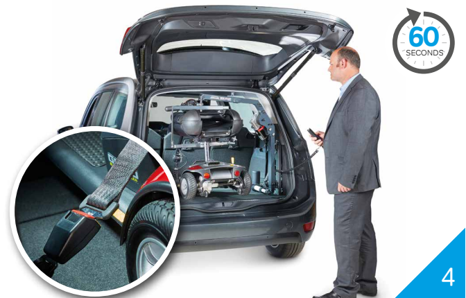
The seatbelt restraint ensures your mini scooter or wheelchair is safely stowed
