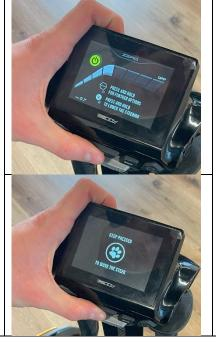
3. Press and hold the "PAW" button to lower the steering shaft
