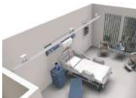
Lifting between two-places with fixed rail (straight-rail system)
