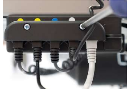
4 | Control box with actuators plugged in
