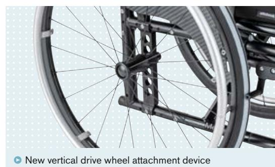
New vertical drive wheel attachment device
