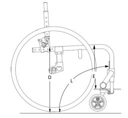
**REAR SEAT HEIGHT D** Measure from floor to top of seat tube at Back Post. Twist adjusts up and down in 1/2" increments.
