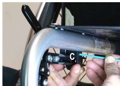
Mark the point where to drill the new hole
