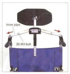
Have a person help by slightly pushing rear handles of wheelchair apart, simultaneously adjust center joints as high as possible (in order to obtain adequate support tension for headrest) then tighten bolts (B)
