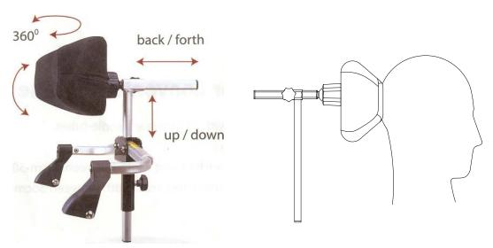
Horizontal position of headrest should be set for occupant comfort within 10mm of head. Height of headrest should be set to centre of occupant's head. The height of the headrest is set by means of a fixing knob as shown in the diagram.
