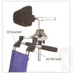
Unfold wheelchair first, loosen bolts (B) to allow inner tubes to slide freely. Fit brackets (E) onto the curved part of push-handles, then tighten bolts (A)
