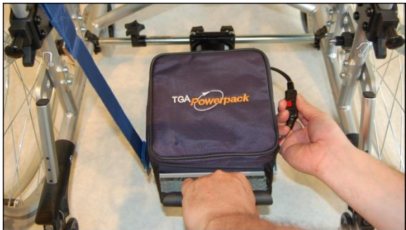
Fig 7 Fitting and Connecting Battery
