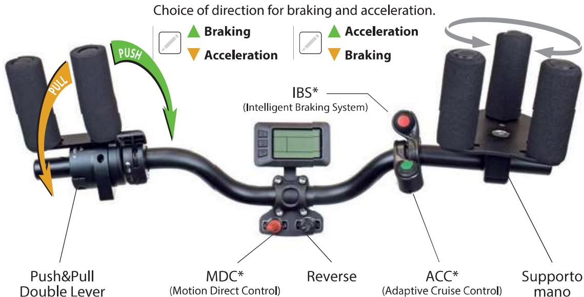
N.B. The triple hand turning supports function is to block the users wrist in order to drive and direct the Triride.
