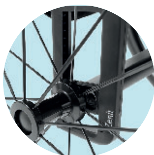
Drive wheel adapter, permanently welded
