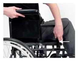
To remove the armrest, press the chrome button at the front of the armrest (arrowed) and pull up on the armrest.
