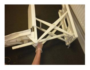
Step 4. Remove the lifting ram and the faulty backrest from the bathlift.
