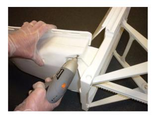
Step 2. Using a T-20 end bit and a screwdriver, remove all the screws on the backrest.
