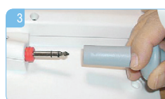
3. Plug the hand control to the bathlift (at the back of the backrest). Make sure that the socket is properly seated on the jack and the red ring on the jack is now hidden.
