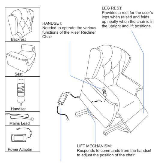
POWER ADAPTER & MAINS LEAD: The chair needs to be connected to a mains electricity supply (220-240V 50Hz) to provide power to operate the rise and recline mechanism.
