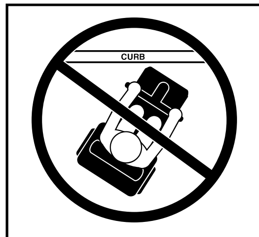
Figure 7. Incorrect Curb Approach
