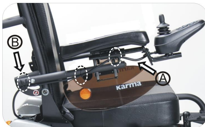
Controller Cable Tie Locations
