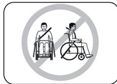
Incorrect seat belt position
