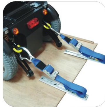
Fitting the rear restraint
