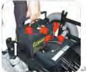
11. Lift up the battery by its handle.
