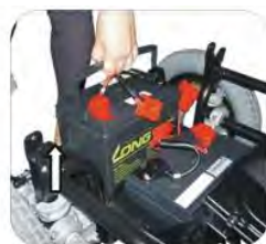
9. Lift up the battery by its handle.
