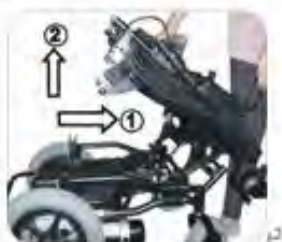
7. Pull the seat forward and upward to lift it.
