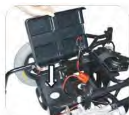
10. After removing the batteries, close the battery box cover.
