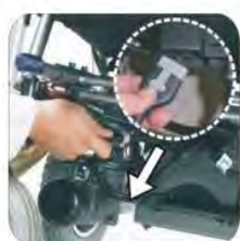
1. Disconnect controller wire.
