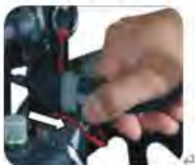
5. Remove the cable from the transmission connector.
