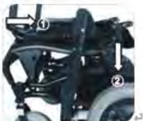
4. Fold the backrest forwards and press it.
