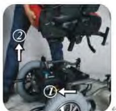
5. Lift and pull the seat backward to remove it from the base frame.
