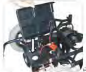
12. After removing the batteries, close the battery box cover.
