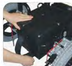
6. Unfasten the Velcro from the bottom of the battery box.
