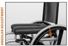
Push the seat max. one pin up on the front of the seat comparing to the back, to create an angular adjustment. Replace the pins at front and push the back down.
