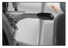
The brakes can be locked or unlocked by pushing or pulling. The brakes can be tighten when needed by using an Allan key nr. 5.
