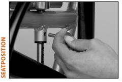
Remove the 4 quick-release pins from under the seat.
