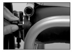
Loosen the knobs of the backrest (left and right) and lay the backrest down.
