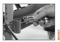
For more adjustment of the leg- and footrests, the legrestreceiver on the frame can be adjusted with an Allan key nr. 4 and spanner nr. 10.
