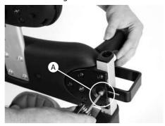
To adjust the height and angle of the lateral supports, loosen the Allen bolt (A), adjust to the required width, height and angle and retighten securely.
