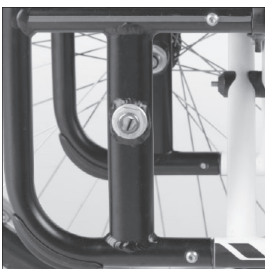
MA 114 Drive wheel adapter, permanently welded
