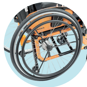
MG83 One-arm drive with double handrim
