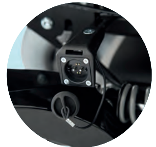
EU043 External magnetic charging receptacle
