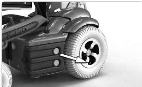
Filling valve, rear tire
