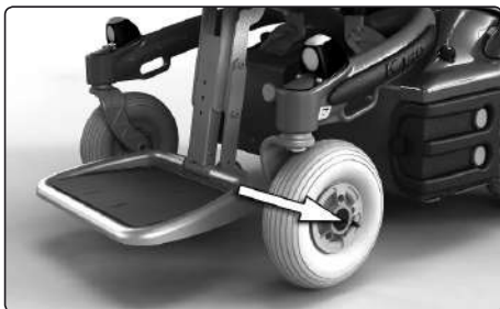
Filling valve, front tire
