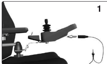
Connecting the emergency operation cable to the charging socket.
