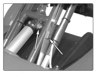
Fig. 38. Fixing screws and catch on cylinder rod
