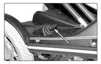
Fig. 27. Releasing the brakes
