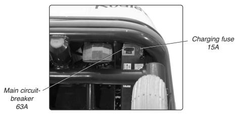
Fig.37. Main circuit-breaker and charging fuse
