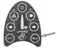
Fig.16. Horn switch
