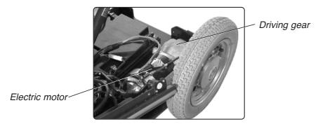
Fig 6. Electric motor with driving gear.
