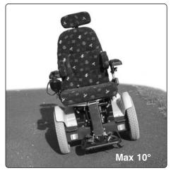
Fig. 30. Driving along slopes
