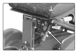
Fig. 2. Seat angle catch when pulled out
