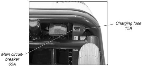
Fig.7. Main circuit-breaker and charging fuse
