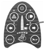
Fig.12. Battery voltage indicator
