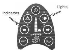
Fig.15. Light/indicator switches
