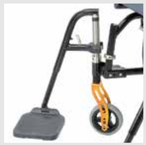
ULM system, for hemiplegic, the wheelchair's directionality is controlled by the footplate that is connected to the fork's axle
