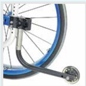
Anti-tip wheel swing away and removable
