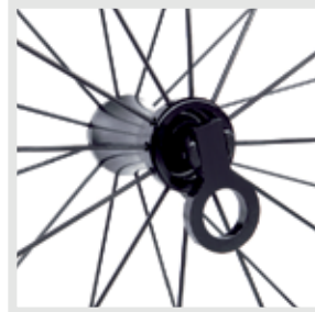
Tetraclip quick release axle for quadriplegic
