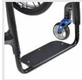
Aluminium footplate with plastic plate
