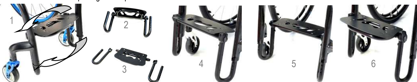
1 Tubes facing backward and footplate forward
