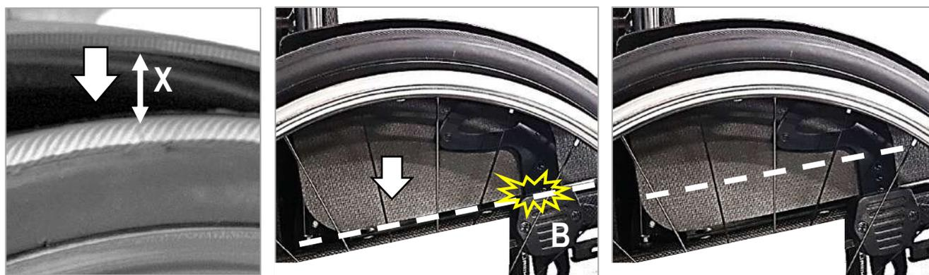
If the lower side of the side guard is in contact with the support, it is necessary to cut it.
