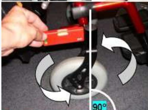
You can now turn the fork support (and the fork itself) clock or anti clock wise within the limits given by the support's slot **A** against the bolt **V**. Within such limits you will have to find the correct angle: the fork has to be perpendicular to the ground.
