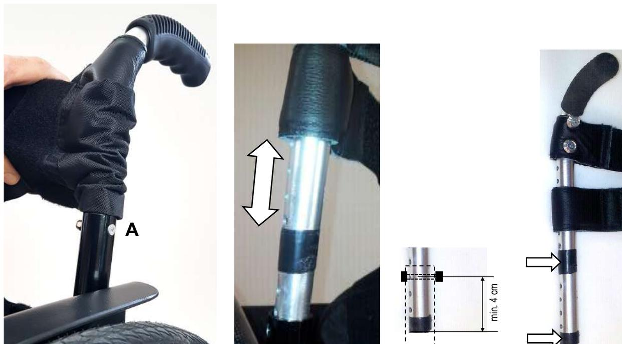
Remove the backrest upholstery and slide up the protecting sleeves of the backrest bands along the tube until the fixing bolt/washer/nut **A** is accessible.
