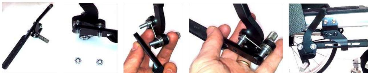
For **sport brake**, remove the two bolts, turn the adjustment rod by 180° and fix the bolts.
