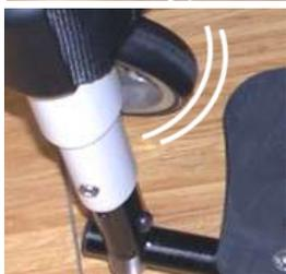
The two white arches show the possible different positions of the fork rotation axis (both at 90° to the ground). The difference can be a few millimetres
