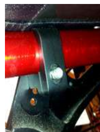
Inner plate of the rear support with embedded nut
