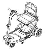
1) Pull the red lever on the floorboard of the scooter to release the lock.
