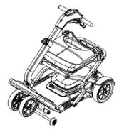
3) Lock the scooter onto the open position by pulling the seat up and pushing the tiller forward until a click sound is heard.
