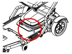
2) Fold the seat backrest down and then fold the tiller downward
