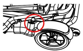
2) Unfold the scooter by pushing the tiller forward
