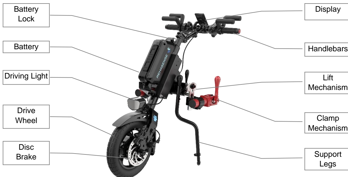
Figure 1. Main Elements for the Device (example shown is manual clamp and lift configuration)
