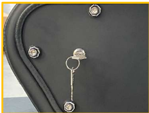
Figure 1 – Speed override switch (ON)
