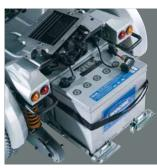
**Easy battery access** Batteries slide out easily for simple servicing. Just open the rear flap gate and pull the batteries out – it could not be easier!
