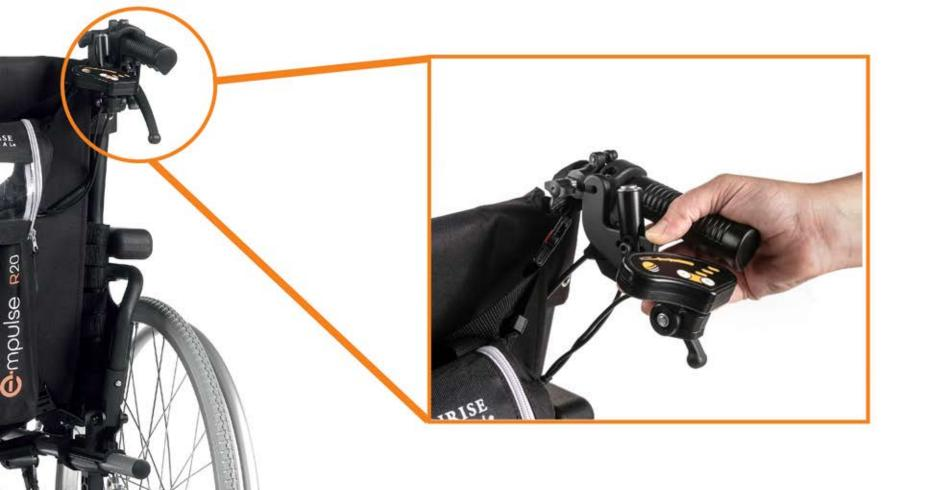
The easy to use control system has **one push button to go,** as well as an easy to read display showing the speed and battery gauges.
