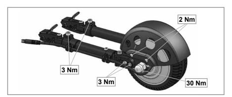
The screws used are fitted with threadlock at the factory and after fitting, cannot be re-used. After that they should be replaced or alternatively re-secured with threadlock to medium tightness.
