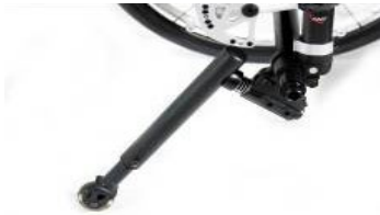
KRR090033 Anti tip flip up (user operated)
