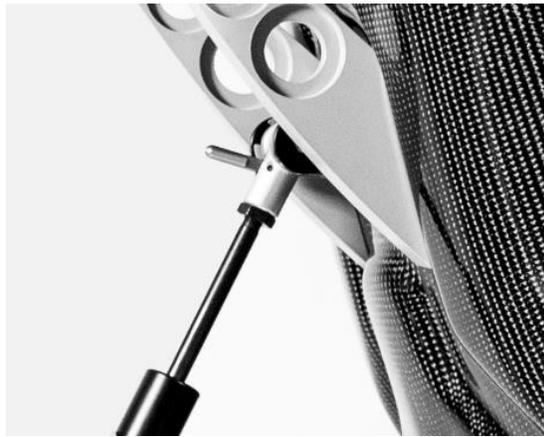
Our patented rear shock absorber helps ensure a smooth ride at all times whilst also acting as a tilt in space mechanism to alter the angle of the seat. This allows you to change the weight distribution in the chair and increase ground clearance as well.
