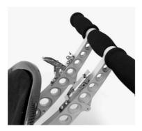
To lock the folding handlebars, first locate the two halves of the handlebar which fit together, then hook the clasp over the catch and pull the clasp back to lock it. This may be a bit stiff but has been designed to be extremely strong to avoid damage. In the above image you can see the nearside clasp locked into position and the far clasp hooked over the catch and ready to be pulled back into the locked position.
