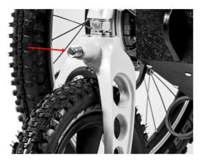
To re-grease, undo the grub screw completely, fill the cavity with general purpose automotive grease and refit the screw, whilst periodically rotating the castor. Repeat until grease is seen appearing from the top bearing. Wipe clean. Regreasing is only normally required at service as stated below.
