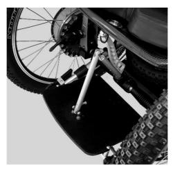
3. Recline the seat by activating the shock absorber and pressing back/down until the shock absorber is fully compressed.
