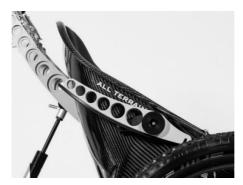
3. Unclasp locks on folding handlebars (not applicable to standard non-folding handlebars) and fold handlebars downwards
