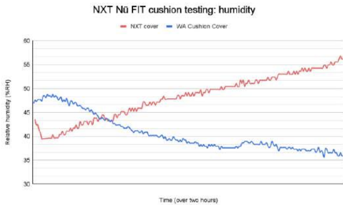
Graph 2. The recorded relative humidity with WA CC was up to 21.2% lower than the NXT cover.
