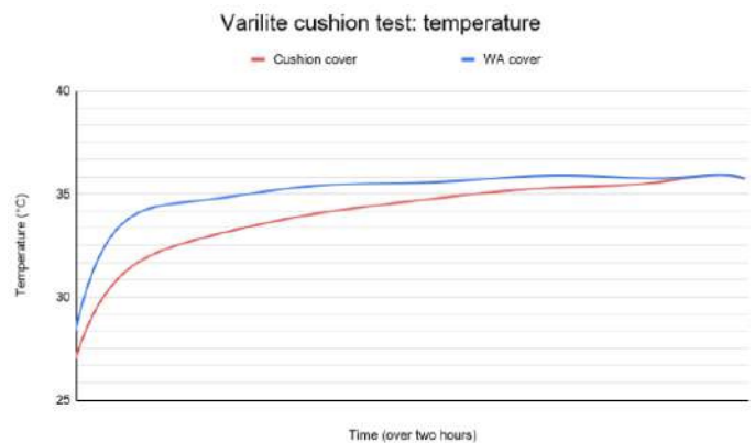
Graph 1. The temperature plateaued up to 0.3°C higher for the WA CC than the Varilite cover
