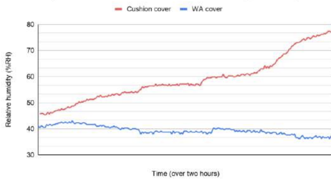
Graph 2. The relative humidity with WA CC was up to 41% lower than the Supracor cover
