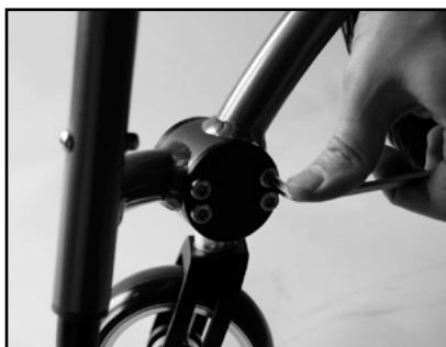
Image 55 Remove the four bolts
