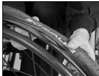
Image 69 Pull out the tube
