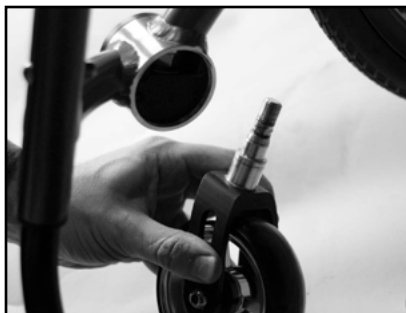
Image 57 Change the caster with front fork
