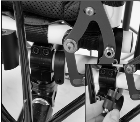
Image 66 Clamp on the frame
