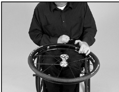
Image 68 Pull the tyre edge over the rim
