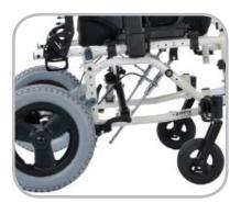
Tilt-in-Space up to 45 degrees. Available in both rigid and folding frames. Also available with Foot Release Tilt Actuator, which eliminates exposed cables.
